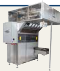
IPP6/22 Intermediate Pocket Proofer with 132 effective pockets, single infeed V-belt conveyor L=750 mm. Photocell controlled, non-stick coated, infeed conveyor combined with continuous pocket proofer drive. Variable speed on the proofer. Electric control panel under projecting overhang, electric sockets for Divider, Rounder and Moulder. Max proofing time 4,3 min at 1800 pcs/h.
