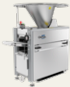
SD180XS Dough Divider with variable speed 500-1200 pcs/h. 90 liter stainless steel hopper. Weight range 50-1000 g.
