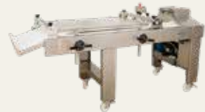
M0300S Moulder with centrally adjustable infeed hopper, curling net and foldable 650 x 1100 mm pressure board. Adjustable side guides and ergonomic collection tray. Operating side right/left.
